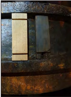
A comparison of the old block and a new one against the pump piston
