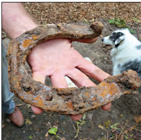
A horseshoe found in the stables area. Our friends at Arraslea Shires (who provide Ted and Chelsea to pull Birdswood) say that the shoe is for a draft horse and looks like it's made of wrought iron with heels to help with grip when pulling. If it is wrought iron it could be 80-100 years old.
