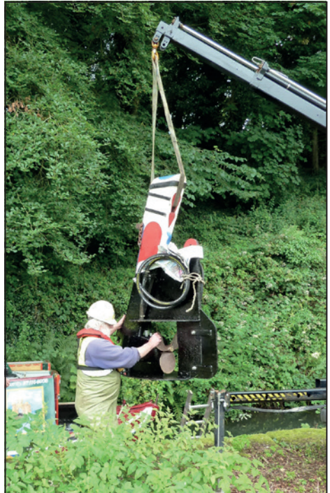
The rudder with new motor and extension plate being lifted back onto Birdswood in July.
