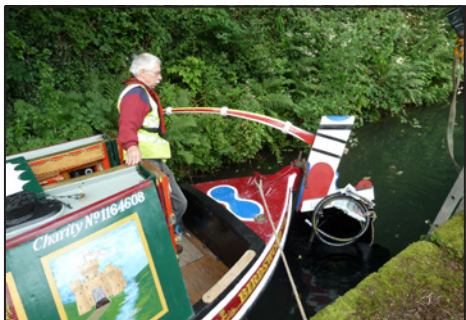
Dave Turner checks the swing of the newly re-installed rudder.
