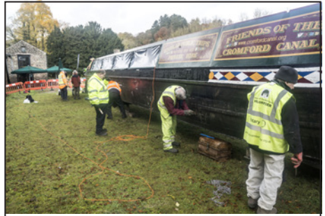
The work party hard at work scraping the hull. Photo: Keith Bailey
