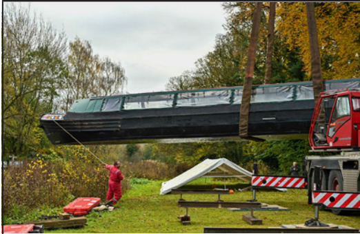
Lift in progress. Walker's banksman steers the hull. Photo: Anne Haile
