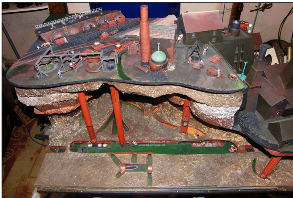
Simon Waller's 00-scale cut-away model showing the Butterley site and the shafts leading down to the Wide Hole below. On the left is the horse gin with the tram box at the top of the left-hand shaft and the counterbalance water bucket at the bottom of the right shaft.
