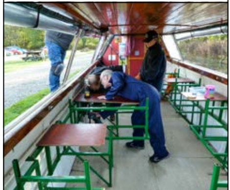
Refixing the new lighter weight seating after an MCA inspection.
