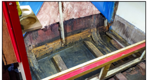
The exposed braces below the bed in the boatman's cabin after cleaning.
