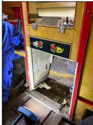
The exposed braces below the bed in the boatman's cabin after cleaning.
