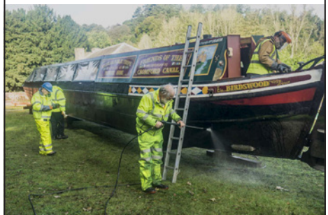
DCC's John Thompson pressure washing the hull.
