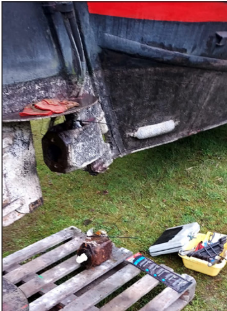
The hydraulic motor removed from the rudder.
