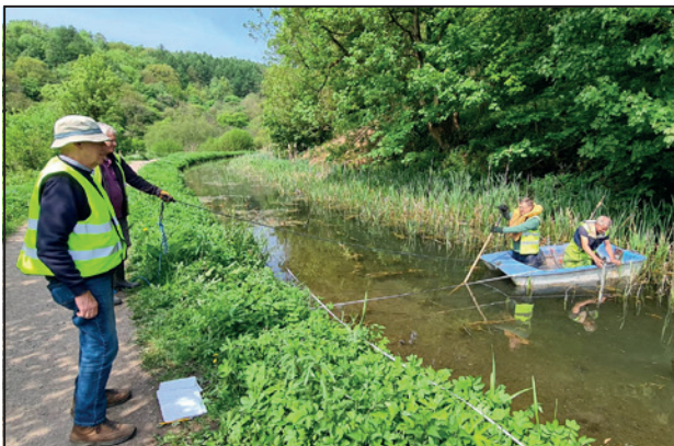
Surveying the canal depth.
